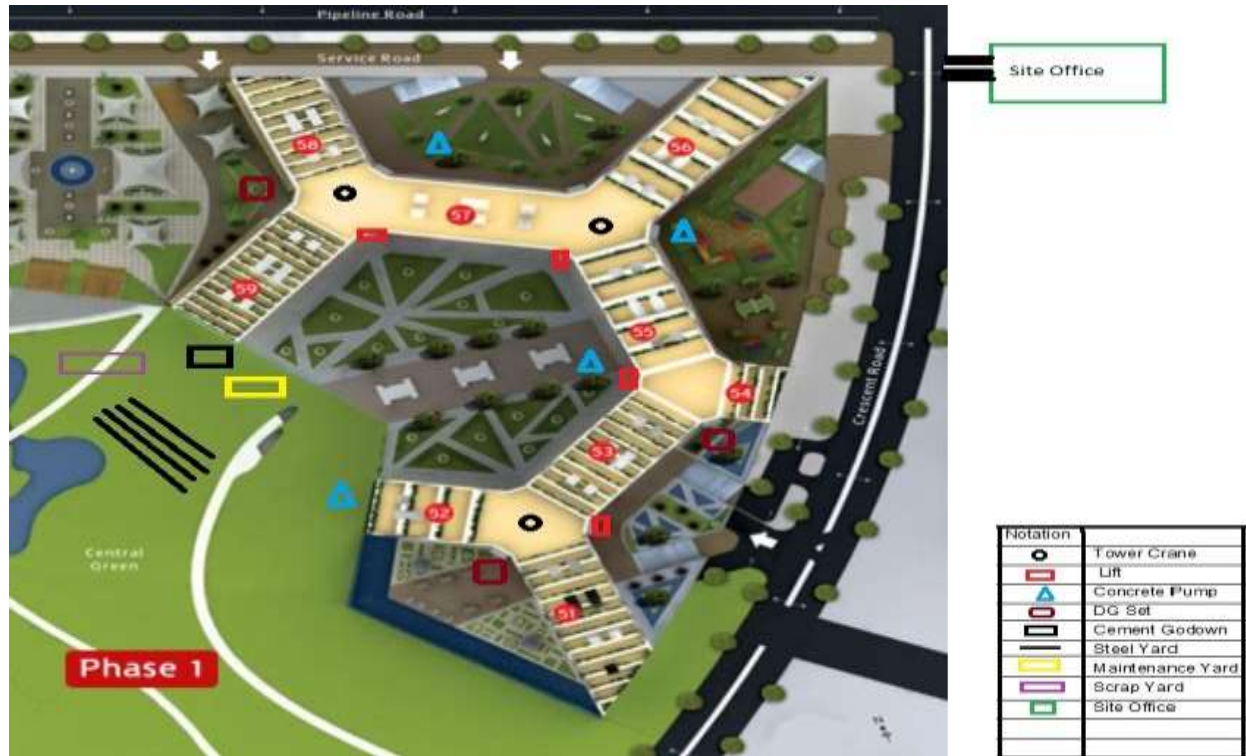
Fig no. 3 Equipment Position on construction site, Pune.
